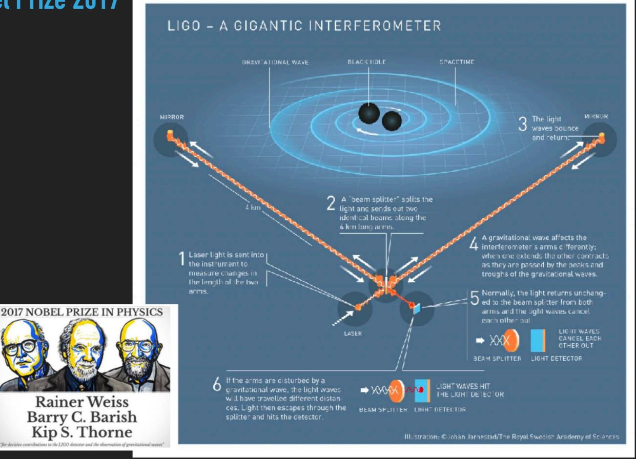
Recall – the Michelson-Morley experiment (looking for the aether) was also an interferometer!
